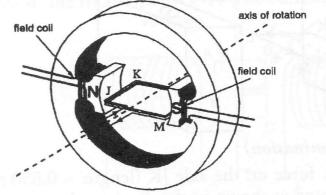
The armature of the motor consists of a rectangular coil with 30 turns. Side JK is 15 cm long and side JM is 10 cm. The magnetic field can be considered to be radial and has a flux density of 0.05 T.
